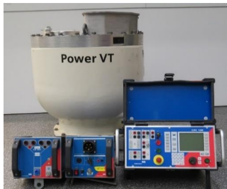
Power VT high-voltage test set-up
